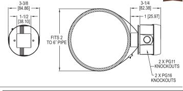
The Series TE-SNW Weather Resistant Surface Temperature Sensor nonintrusively measures the process temperature in hot and cold water loops in buildings. In order to work with most common building controllers, the output of the sensor can be chosen from 6 different RTD and Thermistor curves.
