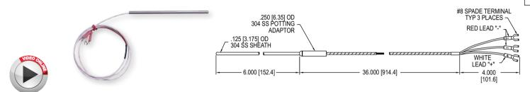
Precision Series RTD Resistance Temperature Detector offers excellent accuracy and stability over a wide temperature range. Industry standard 3-wire 100  $\Omega$  (DIN) probes are available in 6" (15 cm), 12" (30.5 cm), or 18" (46 cm) sheath lengths with 30" (76 cm) extension cable and spade lug terminals.
