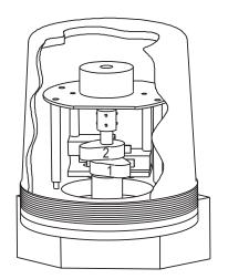
Models 19XXX, 39XXX and 49XXX Rotary Position Indicating Switches contain a 4-20 mA transmitter with HART<sup>®</sup> communication and two Single Pole Double Throw (SPDT) switches. Models 190XX, 390XX and 490XX contain a 4-20 mA transmitter with HART<sup>®</sup> communication only, no switches.
