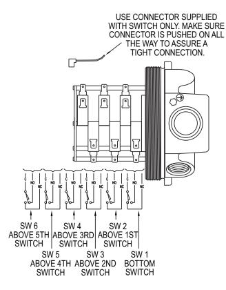
Figure 8: Wiring for switch types B, C, I, R, V, and W. 1, 2, 4, or 6 switches. Switch types B and I have "+" and "-" terminals
