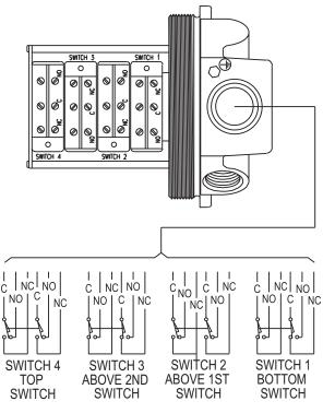
Figure 4: Wiring for switch type D. 1, 2, or 4 switches
