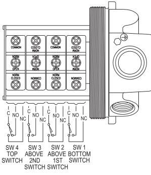
Figure 1: Wiring for switch types A, G, H, M, and T. 1, 2, or 4 switches
