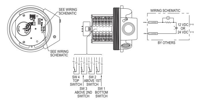
Figure 12: Intrinsically Safe wiring for transmitter with HART<sup>®</sup> communication output. Refer to proper switch figure if unit has switches as well
