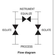
The Series BBV-1 3-Valve Block Manifolds can be used over a broad range of industrial applications including oil refineries, nuclear power stations, petrochemical processing, and more. The Series BBV-1 body is forged from 316 stainless steel bar stock and designed to withstand repeated open and close operations. Suited to control oil, water, toxic fluids, chemicals, air, and steam.
