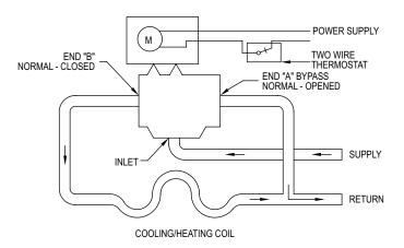
Figure 2: Three-way valve
