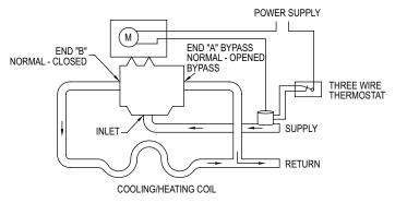
Figure 3: Three-way valve with box change-over switch
