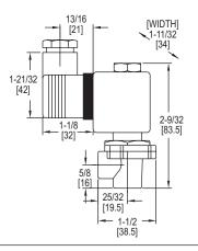
The Series RSV Pilot Solenoid Valve is used to operate the Series RDCV remote type diaphragm valve to air pulse clean filters in dust collectors. Consult factory for mounting of RSV valves with our DCT timer boards together in one enclosure all prewired.
