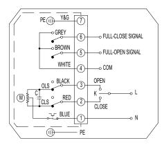
TD02-A to TD07-A: 110 VAC, TD02-B to TD07-B: 220 VAC, TD02-C to TD07-C: 24 VAC
