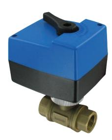
The Series HBAV is an electrical ball valve ideal for flow control in hot and cold water HVAC systems. These valves are typically used in conjunction with air conditioning systems, heating systems, water treatment and production industries. The HBAV is electrically driven open and/or closed via a bidirectional AC motor. The electrical valve offers a detachable actuator with position switches and indicator. The HBAV is available with modulating or floating actuators.
