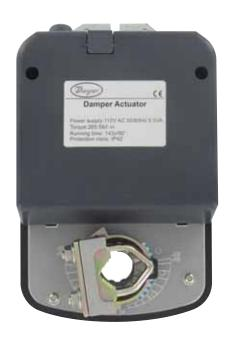
DDD Series Direct Coupled Actuators are non-spring return actuators that are perfect for positioning of dampers and valves in HVAC systems. Actuators are designed to accept 4 to 20 mA or 0 to 10 VDC modulating control signals and are 24 VAC powered. Actuators produce 88 to 265 in-lb (10 to 30 Nm) of torque. Unit features a 0 to 10 VDC feedback signal of damper position.
