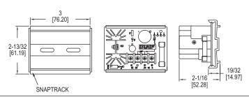
The **Model BPS-005 Low Cost DC Power Supply** is a regulated .5 A power supply that accepts 24 VAC input and provides an adjustable 1.5-29 VDC output. Output voltage adjustments are made using the on-board potentiometer while measuring the output with a multimeter. A compact snap track design allows the power supply to be surface mounted within a panel.
