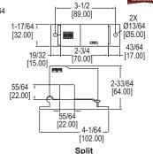
The Series CCT40/50 Current Transformers are a low cost alternative for measuring power and monitoring the operation of fans, pumps, or other equipment. For use on existing installations, split core models can be installed without disconnecting cables. Each model offers three jumper selectable ranges and a choice of three different outputs.
