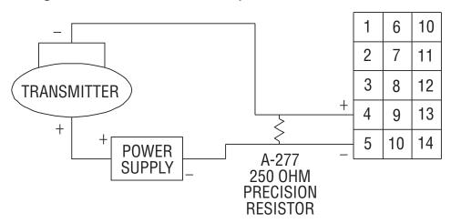
Note: 16B terminal layout used in above example. Use appropriate terminal layout for selected controller.
