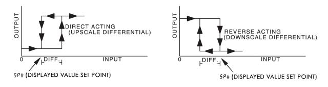
Figure A: Output behavior for Heating/Cooling On/Off Applications
