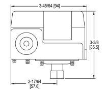
The **SERIES CXA** Water Pump Pressure Switches have been proven reliable for controlling automatic water systems. These switches are very popular for use on water well pumps and pumping systems. The set point and deadband are both easily adjustable via screws inside the cover. For ease of installation, the switches come with a 1/4" female NPT process connection and can be mounted in any orientation. The series CXA's simple design makes it a great switch for an installer at any skill level.
