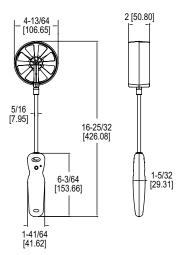
The **Model VP3 Wireless 100 mm Vane Thermo-Anemometer Probe** measures air velocity, air flow, humidity, and temperature with the UHH4 or newer universal handheld device, or your own mobile device. By having a larger diameter, the rotating vane is able to measure velocities down to 50 FPM or 0.25 m/s. An arrow is molded into the vane housing to depict the flow direction.
