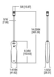
The **Model RP3 Wireless Thermo-Hygrometer Probe** measures relative humidity, temperature, dew point, and wet bulb temperatures when combined with the UHH4 or newer universal handheld device, or your own mobile device. In order to protect the sensor in higher air flow ducts, each probe comes with a membrane filter. Factory calibrated replacement humidity sensors can plug directly into the probe without requiring additional calibration.
