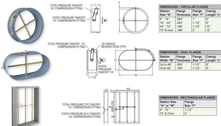
The Series FLST Duct Mounted Airflow Measurement Stations utilize an airflow averaging element generating a velocity pressure signal similar to the orifice, venturi, and other primary elements. Single or multiple airflow elements are factory mounted and pre-piped in a casing designed for flanged connection to the ductwork. Multiple elements are joined together for connection to a differential measurement device (gage, transmitter, etc.) for flow measurement and indication purposes.
