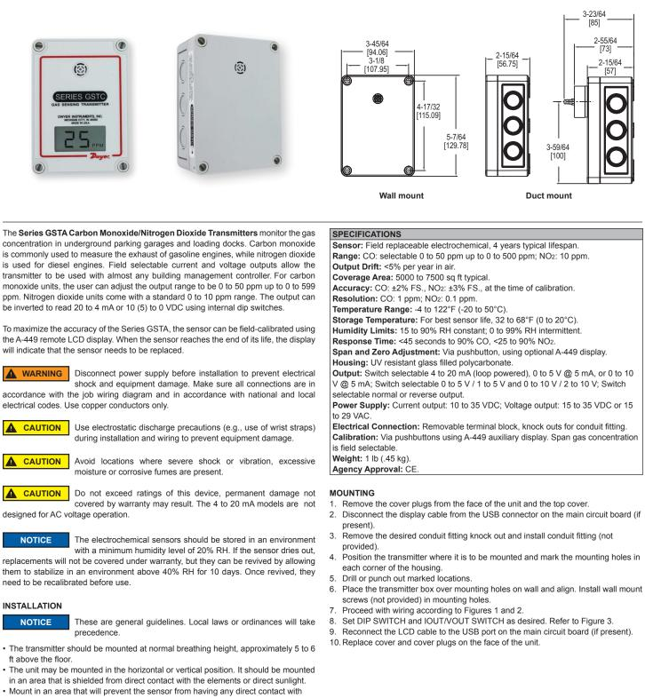
water.The unit should be placed in an area that will give an average of the air quality. Do not place the unit so it will receive direct engine exhaust. Prolonged exposure to
