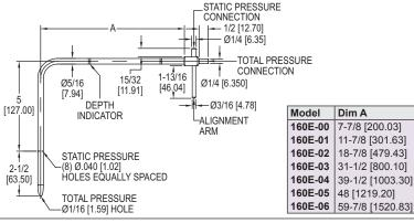
The Series 160E Ellipsoidal Tip Pitot Tube uses a precision crafted tip configuration, which allows air to pass smoothly with minimum turbulence for consistent, reliable readings. Sliding depth indicators grip firmly to ensure uniform insertion when measuring traverses across ducts. Total and static pressure taps are 1/4" (6 mm) and are permanently silver soldered to the connection block, making them leak-proof and durable
