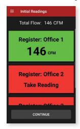
Repeat this procedure until all of the registers have been measured. Clicking on a register again allows for a retaking of that register if needed.
