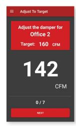
"Manual Data" will bring up the Manual Data screen similar to the initial sweep manual entry dialog. After the manual data is entered, another dialog will appear. This manual entry dialog asks for the flow of the register after adjusting (if it can be adjusted). The dialog includes the target flow that the register needs to reach to balance the system.
