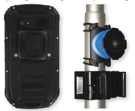
Once the handheld is attached to the pole, the SMART Air Hood® balancing instrument is now ready for use.
