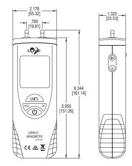
The MODEL LDPM Digital Differential Pressure Manometer is a versatile, handheld, battery operated manometer that can measure up to 55.4 in w.c. (140.6 cm w.c.). It is able to measure either positive, negative, or differential pressure with a  $\pm 3\%$  FS accuracy. Users are able to select from 11 common English and metric pressure units.
