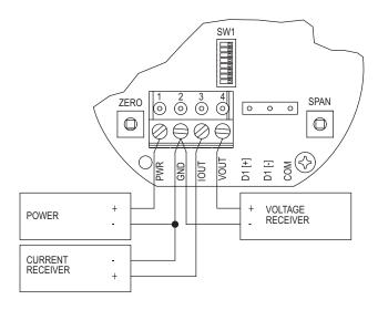
Figure 3: Simultaneous current and voltage output wiring
