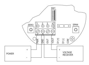
Figure 2: Voltage output wiring
