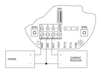
Figure 1: Current output wiring
