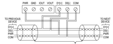
Figure 7: Common power supply
