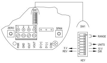
Figure 4: Analog DIP switches
