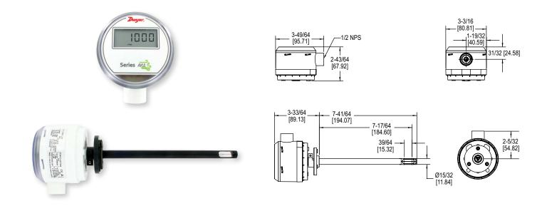
The Series AVUL Air Velocity Transmitter quickly and accurately measures air velocity or volumetric flow in imperial or metric units. Simultaneous current and voltage outputs on all models provide universal inputs to monitoring equipment while the output range, units, and 0-5/10 VDC output can be configured via local DIP switches. The optional integral display, or the portable remote display tool, provide a convenient way to locally monitor process values and configure the unit.
