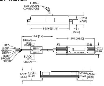
The Series UBT Clamp-On Ultrasonic Thermal Energy Meter is an economical clamp-on ultrasonic heat meter. It is an ultrasonic alternative to the traditional inline thermal energy meters. The series uses temperature sensors for energy measurement and ultrasonic waves with time differentials for flow measurement.
