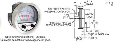
[4] 6-32 HOLES EQUALLY SPACED ON A 5-1/8 [130.18] B.C. 0 ø4 [101.60] FACE
