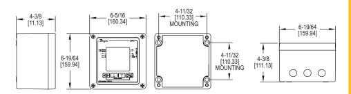
The Series DPM Particulate Monitor & Control and Series PMS Particulate Sensor combine to provide a basic baghouse and cartridge filter leak detector designed for general maintenance planning and process protection. Leakage is gauged in realtime, on-the-spot, without prior baseline data and without signal tuning and displayed on the digital readout in a bar graph and an absolute digital readout. An alarm point can be set by simply moving an indicator up and down the gauge with the key pad.
