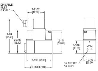
The Series 629HLP Differential Pressure Transmitters are suitable for measuring over-pressure, under-pressure, and differential pressure in compatible gases and liquids with 1% accuracy. The 629HLP is suitable for all measuring tasks in commercial, industrial or sanitary applications. Its single sensor design, allows it to measure small increment pressure changes, and converts them to a linear analog output signal from 4-20 mA or 0-10 VDC.
