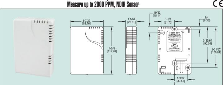
The Series CDW Wall Mount Carbon Dioxide/Temperature Transmitter combines accurate CO2 measurements with a passive temperature output. The Non-Dispersive Infrared (NDIR) sensor continuously updates the calibration through a proprietary logic feature which limits the amount of error due to drift. The CDW series is ideal for building automation systems to help control the fresh air intake in a room.
