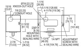
Reliable and convenient, the Series AP Diaphragm Operated Pressure Switch is a compact switch for instrument air or other low pressure applications. Visible set point and external adjustment add convenience. Used on air, non-corrosive gas or liquid service compatible with wetted parts. Units are available in weather-proof and explosion-proof housing.
